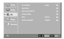
Tuner Mode : Antenna (over-the-air broadcasts, Ch 2-69) or Cable (cable/satellite broadcasts,
